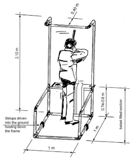
Shooting position in coloured 50mm diameter PVC tubes Straight tubes + interlocking elbows. All of the lower part to be filled with water or sand or fixed to the ground.
